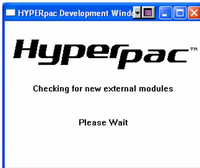
Once the scan is complete the HyperPAC will display the list of all new modules that were detected. Note that several modules can be scanned in at the same time. Also note that once a module has been scanned it will not show up on future scans for new modules. It will only be displayed on the Review Modules screen.
